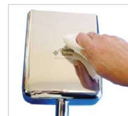
4. Clean etching area thoroughly using demineralised water
