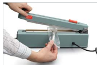
Seal the open end of the bag
